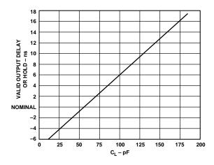
Figure 18. Typical Output Valid Delay or Hold vs. Load Capacitance,  $C_L$  (at Maximum Ambient Operating Temperature)
